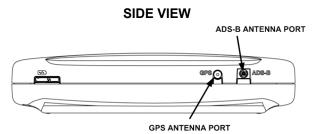
**WARNING:** Ensure you are connecting the antenna to the correct port.
